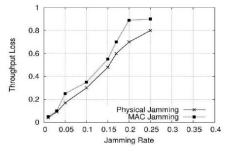
Fig 5 (b) Effect of Jammer Rate on Throughput loss
