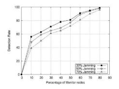
Fig 5 (f) Impact of monitor node ratio on detection rate
