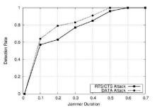
Fig 5 (d) Impact of jamming duration on detection rates
